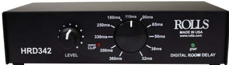
CLIP LED: Indicates that the amount of signal is above a normal operating level.
