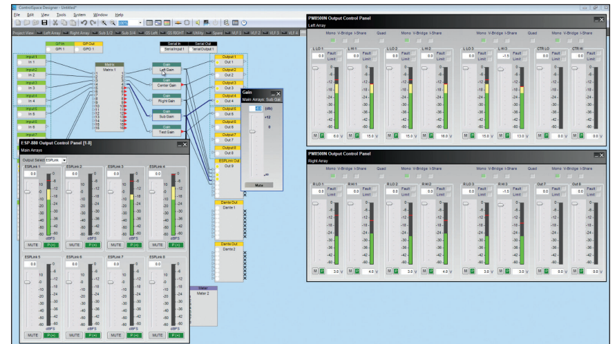
Real-time network monitoring of multiple amplifiers
