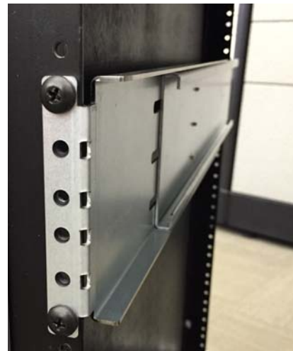
Figure 4. Outer Rack Support attached to the front-left rack rail
