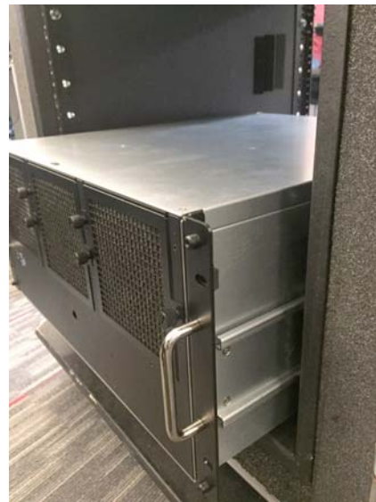
Figure 7. Sliding E6L into an enclosure
