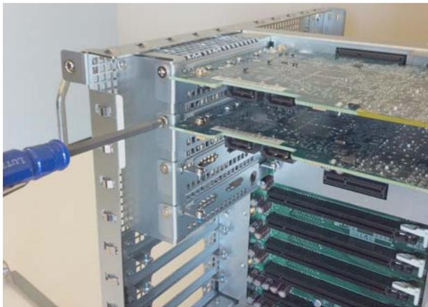
Figure 10. Tightening the front bracket screw
