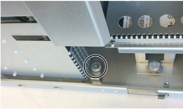
Figure 4. HDX card Bracket thumbscrew
