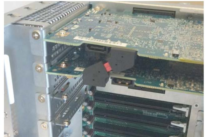
Figure 12. Properly Connected Flex Cable
